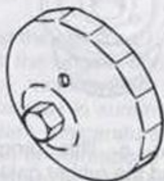
Oil filter wrench (Part No. 09915-40610)
